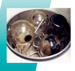
清洗之前 清洗容器内受沥青污染的烧瓶 **Wash container** with polluted flasks before washing process
